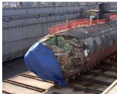
USS San Francisco in dry dock to assess damage sustained after running aground approximately 350 miles south of Guam. Photo by Mate 2nd Class Mark Allen U.S. Navy
